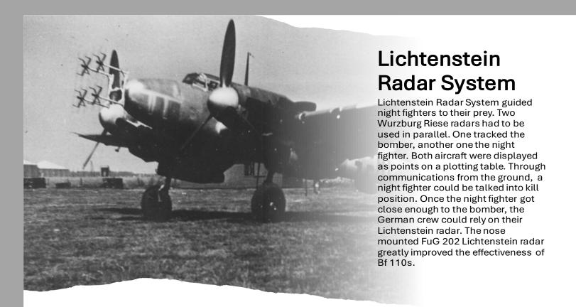
FuG 202 Lichtenstein radar fitted to Bf 110 G-4 (c.1942).
